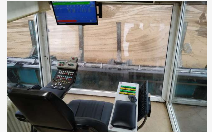
Log sorting control system
